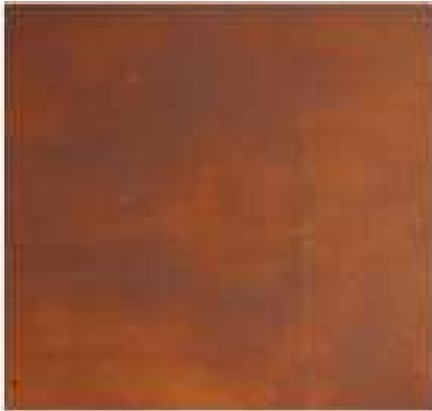
COR-TEN Steel Panels at walls and planters
